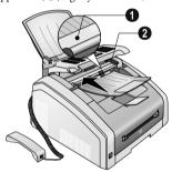
3 Clean the rubber roller of the document feeder (6 x) with a soft lint-free cloth. Rotate the feed roller; You must clean the entire roller.
