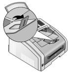
**3 Printing on A5 Paper:** Fold the print out support with the pulled out paper stopper back again.
