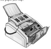
**6** Place the toner cartridge into your device. The cartridge should snap securely into position.
