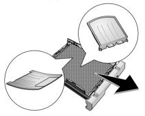
**4** Removing the tape in the paper tray which was used for transportation purposes.
