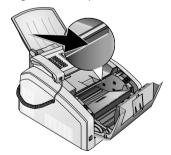
**4** Place the toner cartridge into your device. The cartridge should snap securely into position.
