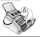
2 Remove the toner cartridge by gripping the handle in the middle and pulling it forwards out of the device
