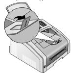
**2 Printing on A5 Paper:** Fold the print out support with the pulled out paper stopper back again.
