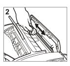
Clean the glass surface of the optical reader with a cloth dampened with a product designed specifically for cleaning glass and then dry it thoroughly.
