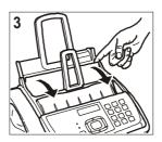
Open the automatic sheet feeder (ASF) panel as indicated by the arrows.
