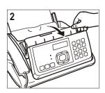
Lift the print cartridge compartment cover using the lever. To release the print cartridge, loosen the strap.
