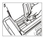
5. Clean the electrical contacts of the print cartridge carriage with a slightly damp cloth.
