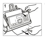
Open the console, remove the document from the ADF and close the console again.
