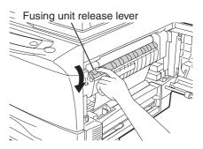
Gently remove the misfed paper from under the fusing unit as shown in the illustration. If the paper cannot be removed, proceed to "C: Misfeed in the transport area".
