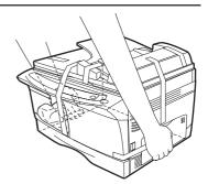
Remove all pieces of tape shown in the illustration below. Then open the original cover/SPF and remove protective materials. After that, take out the bag containing the power cord and TD cartridge.
