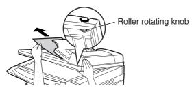
(C) If the original does not move easily into the exit area, remove it in the direction of the arrow while rotating the knob.
