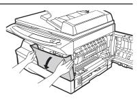
Remove the TD cartridge from the bag. Remove the protective paper. Hold the cartridge on both sides and shake it horizontally four or five times. Hold the tab of the protective cover and pull the tab to your side to remove the cover.
